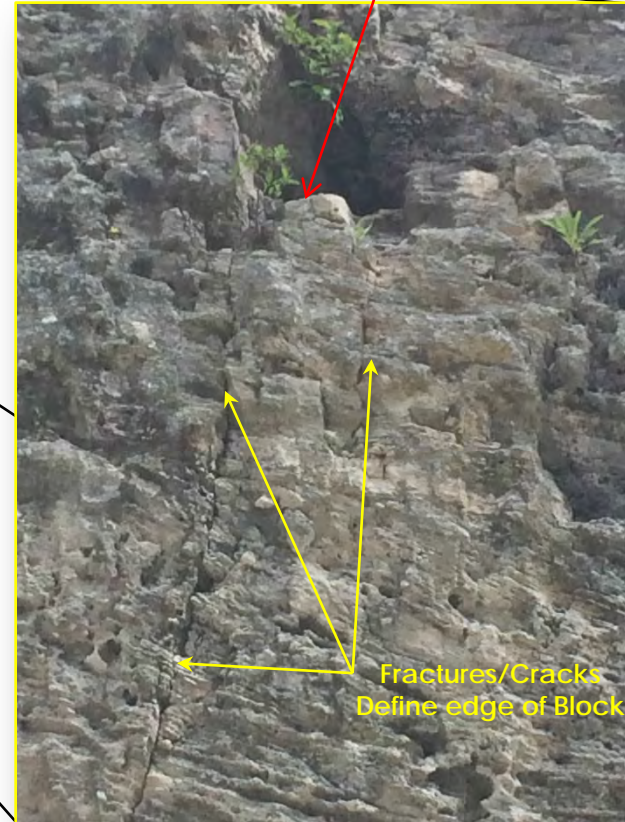
FIGURE 4 PHOTO SHOWING FRACTURES OR CRACKS IN ROCK FACE GIVING RISE TO POTENTIALLY UNSTABLE ROCK MASS/BLOCK
